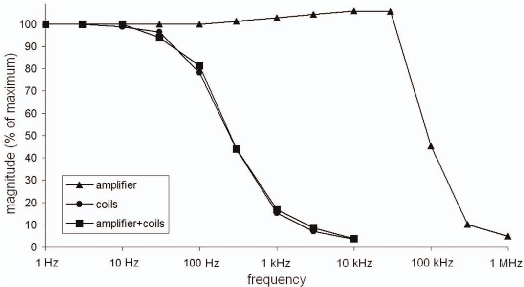
**Figure 3. Frequency characteristics of amplifier, coils and amplifier + coils.**
