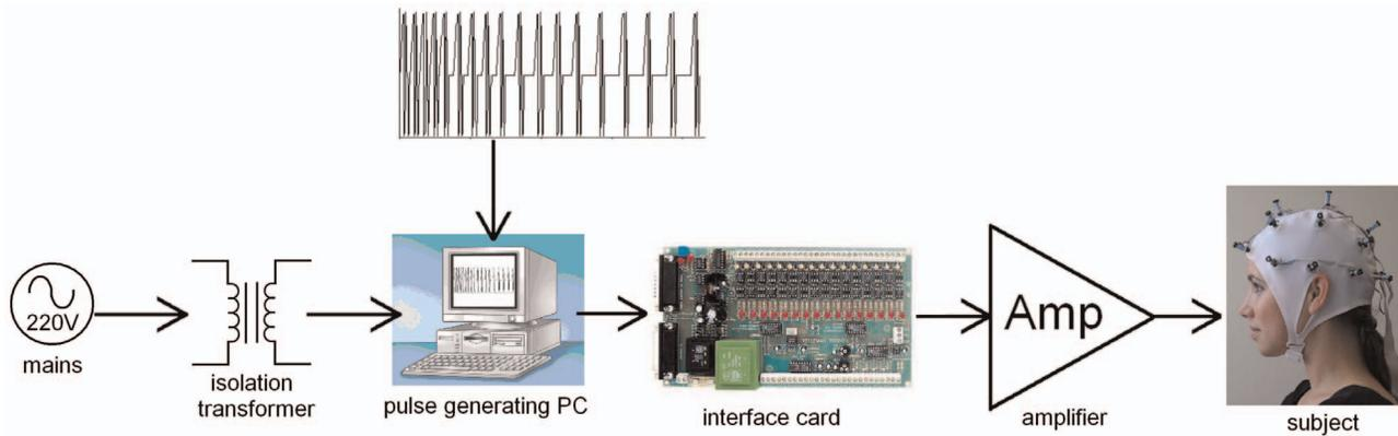
**Figure 1. Schematic overview of the hardware.** The interface card translates digital values into voltages. The amplifier in turn increases power to generate pulsed magnetic fields in nineteen small electromagnets radially attached to the head cap. Photo by S. Martens, consent to publication was obtained from the subject.
