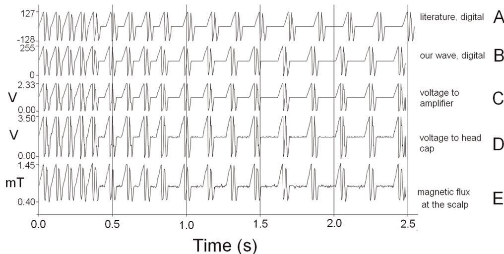
**Figure 2. Different stages of the CNP signal.** The digital version of the CNP wave as published in the literature[22] (A) and used here (B), was converted by PC and interface card to the analogue version (C), which was amplified (D) and converted to a magnetic wave (E), all to the same time scale.
